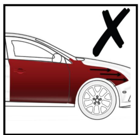
6. 2K tinted clearcoat should cover and overlap the base-coat application area and then blended in to out to avoid arching. It is essential not to coat the whole repaired panel with 2K tinted clear especially the part facing the adjacent panel mostly to avoid darker shade and therefore color difference to adjacent panel. After application and blending of 2K tinted clearcoat.
