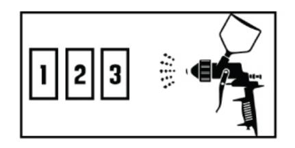
Apply the correct colored primer, as given by Hymix, to 3 test panels and flash-off or dry properly.
