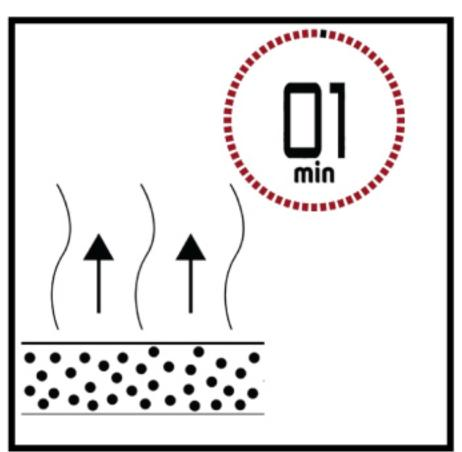
8. Allow no more than one minute flash off in between the tinted and the un-tinted clears to melt down the resulted overspray on the opposite edge of the repair area.
