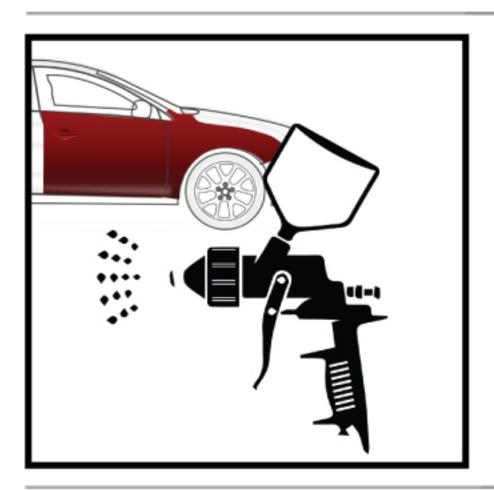
7. Apply one coat of the same clearcoat in use in its non-tinted version to the whole panel(s) to blend in the repaired area and to achieve the best results.
