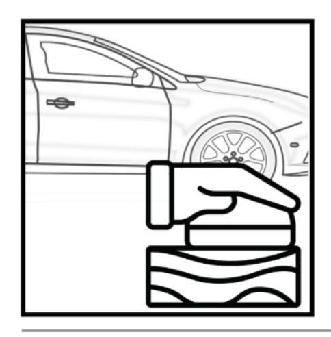
After a good preparation to the repair area, flat the whole panel with P1000-P1500 dry or P1500-P2000 wet to ensure good adhesion and to avoid dark arches.
